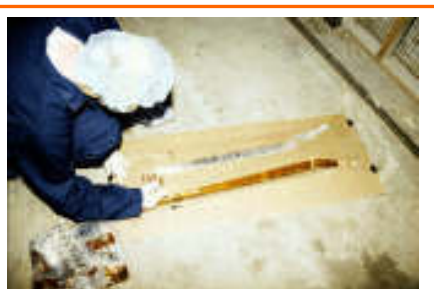
Nuisance flies captured on fly tapes are protected with plastic wrap to be counted back at the laboratory
